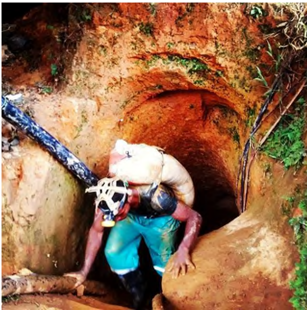
Figure 2. Lack of proper safety equipment creates a dangerous work environment for illegal miners who often climb down into narrow mine shafts without a harness or sufficient lighting, as this miner is doing at Mina Estrella de Orión in Segovia.
